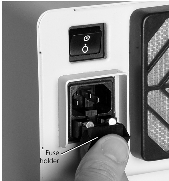
Figure 8-4. Replacing a fuse
