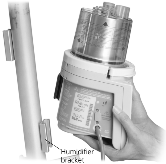
Figure 2-3. Installing the humidifier
