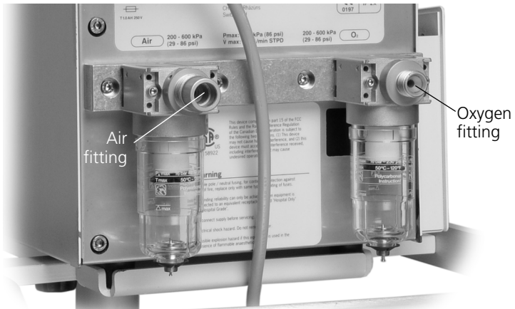
Figure 2-2. Connecting the air and oxygen supplies
