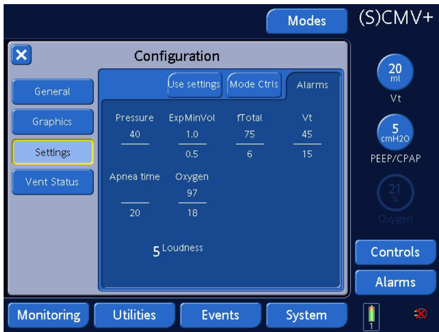
Figure I-7. Alarms configuration window
