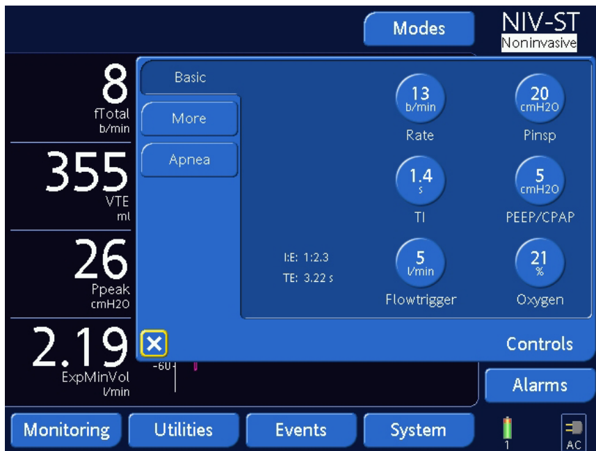
Figure B-23. NIV-ST basic controls
