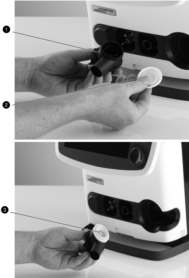
Figure 2-6. Installing the expiratory valve
