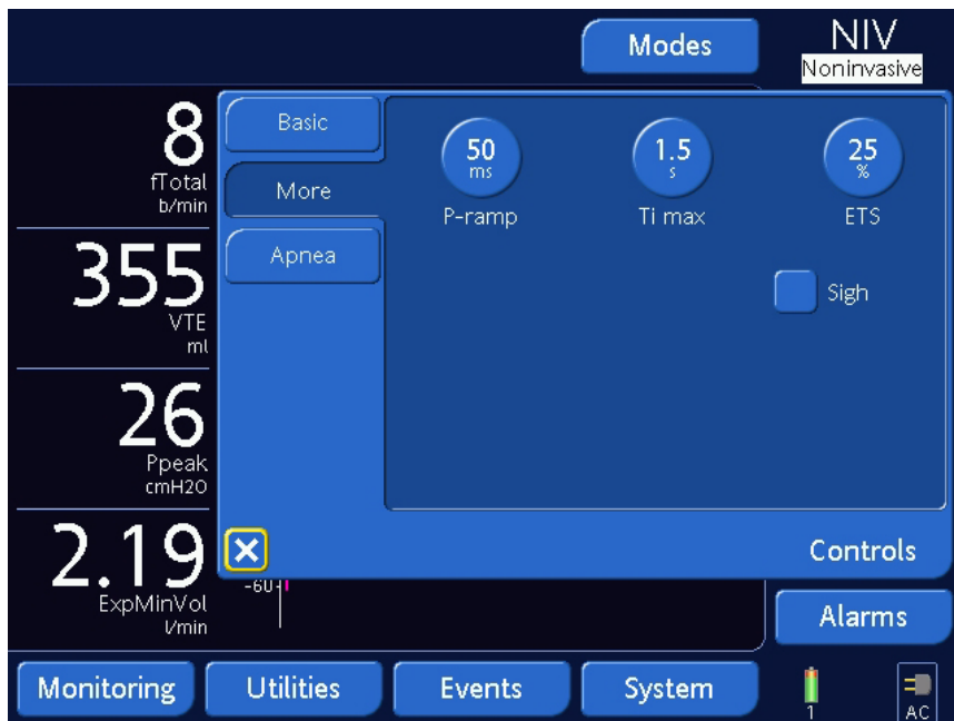
Figure B-13. NIV more controls
